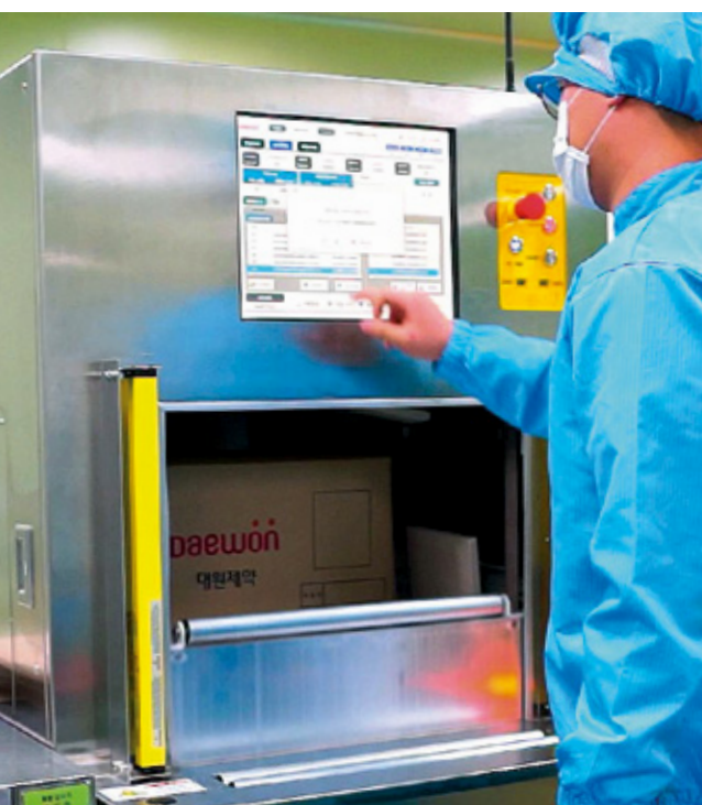
The RFID Bulk Reading Machine is available in two variants: one for manual operation (left) and one for use on conveyor systems (above)
