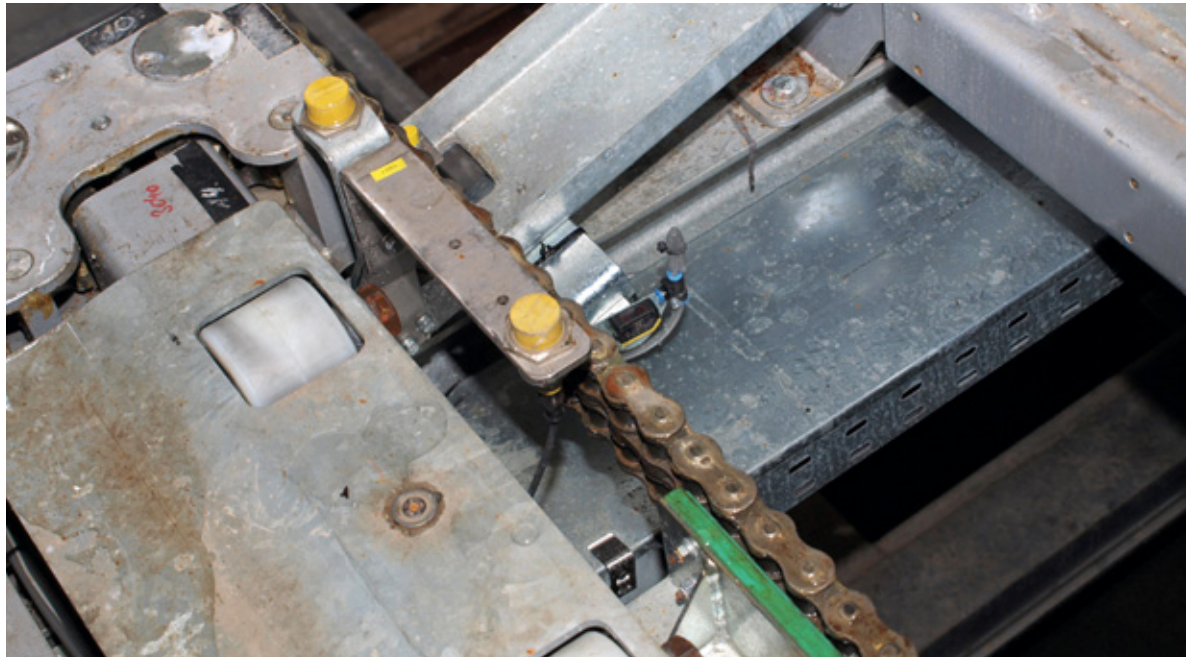
Inductive sensors from Turck monitor the entire berthing and unberthing of the boats
