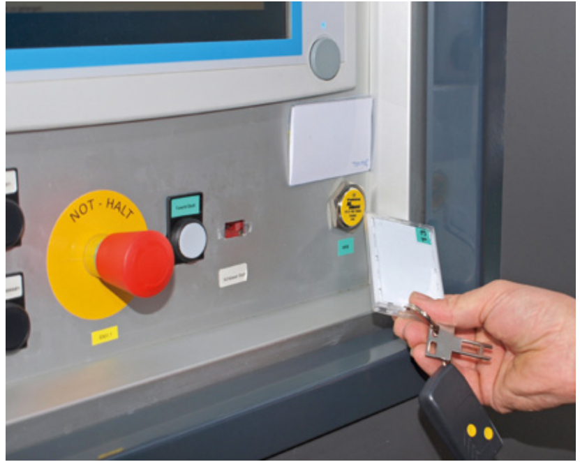
The renter logs in with his RFID chip card on the control panel – the boat is then “delivered” ready for boarding within a few minutes
