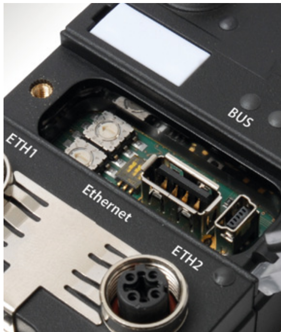
The USB connection is used as a memory interface or for transferring data or software to the device
