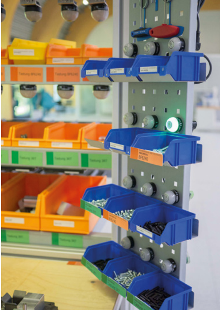
The small K30 lights are ideally suited to incorporating the C parts containers
