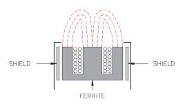
Embeddable construction includes a metal band that surrounds the ferrite core and coil arrangement. This helps to "bundle" or direct the electro- magnetic field to the front of the sensor. Figure 3
