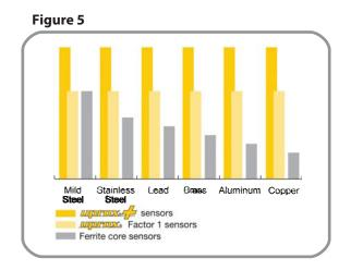
Operating distances comparison of Uprox sensors and standard inductive sensors.
