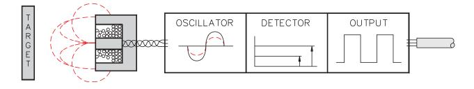
An inductive proximity sensor consists of a coil and ferrite core arrangement, an oscillator and detector circuit, and a solid-state output (Figure 1). The oscillator creates a high frequency field radiating from the coil in front of the sensor, centered around the axis of the coil. The ferrite core bundles and directs the electro-magnetic field to the front.
