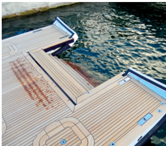
When the platform with the boarding ladder is deployed, the inclination of the platform must be measured in relation to the ship
