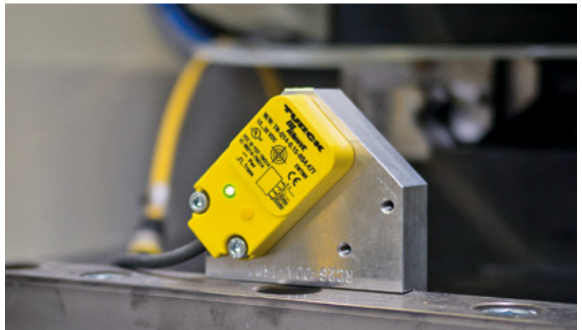
Kirschenhofer chose the TN-Q14 read/write head with IP67 protection due to its compact design
