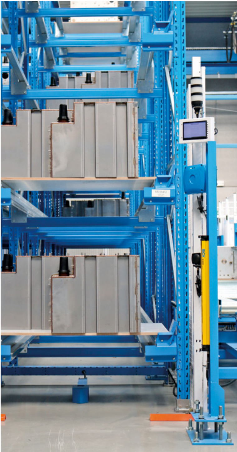
A read/write head also records products when they are checked in and out of the internal warehouse
