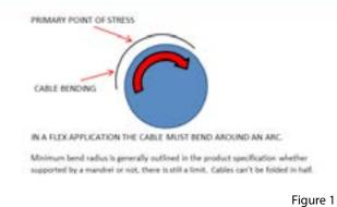
As shown in *Figure 1*, when a cable flexes, it bends around an arc. Now, when the arc becomes larger around the center point, there is a greater distance.
