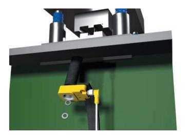
No matter what type of sensor is used, the signals that are created must be sent back to a controller so it can take the appropriate action to protect the die. This is accomplished via wires and cables. Some sensors have cable or wires running out of the sensors that can be directly wired to the controller, while other sensors have
