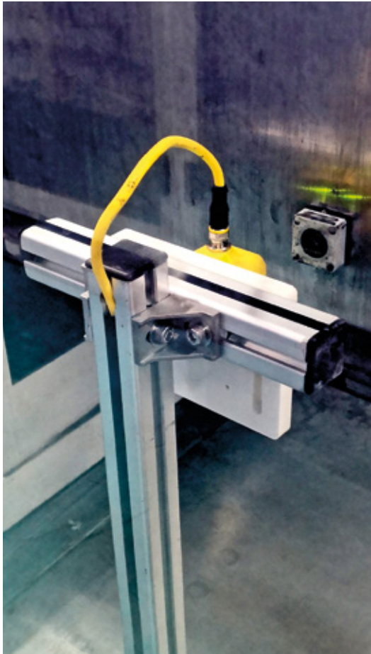
HF read/write heads at each process station ensure reliable data acquisition
