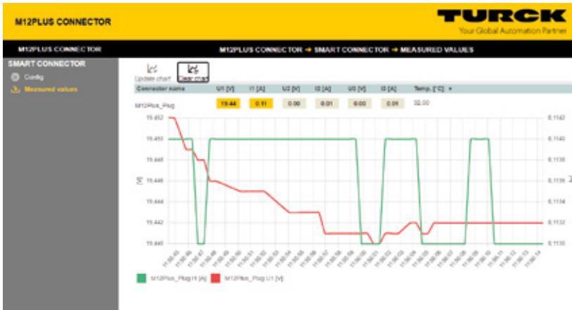
The Turck Automation Suite graphically displays the measured values of the M12Plus
