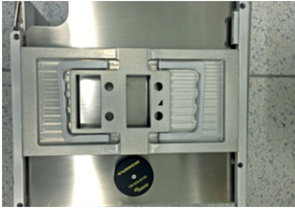
The RFID tag is located on top of the wafer carrier
