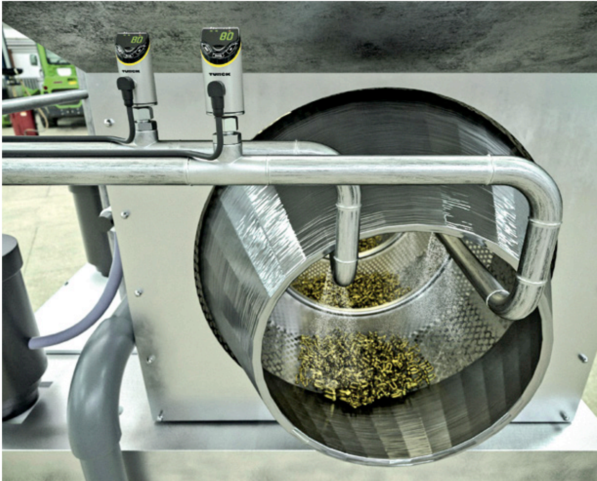
Drum washing plant example: The robust FS+ flow sensors monitor the flow rate and temperature of liquid media
