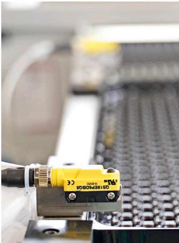
A QS18 photoelectric sensor detects the tray on which the finished connectors are placed
