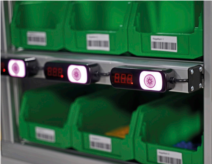
Turck's pick-to-light devices and brackets of the Banner PTL110 series can be used easily without the need for additional tools or reprogramming
