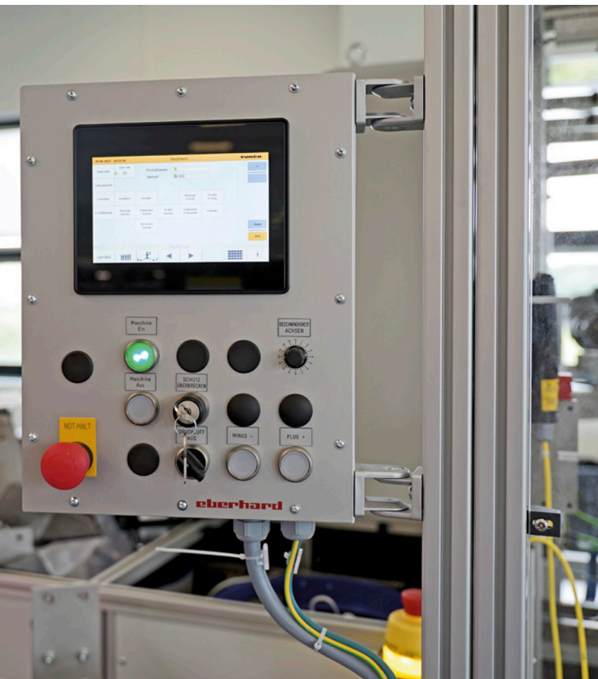
A Turck HMI from the TX700 series is used for visualization and cloud connection
