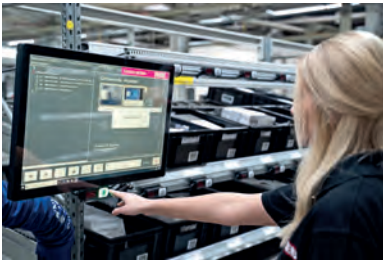
The software brings illustrated instructions onto the screen, the operation is confirmed using capacitive touch buttons
