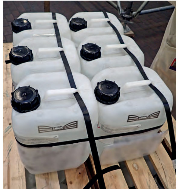
Polar liquids like ethanol are also reliably detected if the tag is positioned correctly
