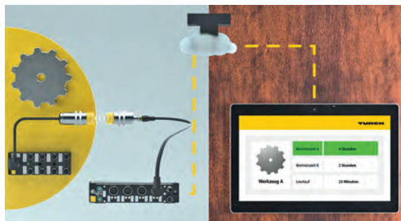
Users can conveniently see in the cloud dashboard the operating hours of each individual tool
