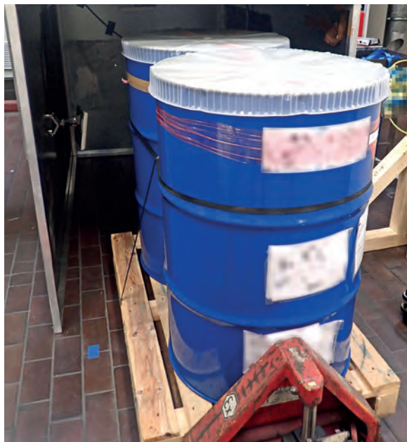
In this case the on-metal tags use the drum itself as an extended antenna
