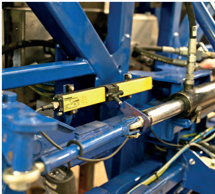
Thanks to its robust design and IP67 protection, the LI500-Q25 inductive linear position sensor can also be fitted outside above the front axle, in order to measure the piston position of the steering cylinder
