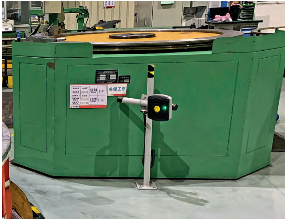
A programmable gateway in Turck's BL20 I/O system controls the decentralized RFID readers – a great benefit considering the large number of production stations in the company
