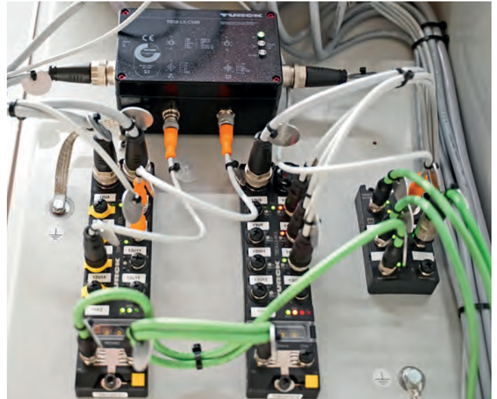
This safety application is controlled by the TBNP (left) for testing in the factory. A Profisafe controller then takes over the application in live operation at the end customer. All actuators connected to the IO-Link master (middle) are safely disconnected with the TBSB Box (above)
