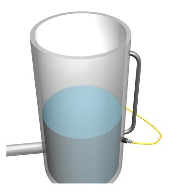
This same theory can be applied in a level application. If a tank is filled with liquid, the same downward force is being applied to the bottom of the tank. The amount of liquid weight, along with gravity, is creating a deflection to the bottom of the tank. With some quick calculations, the amount of liquid in the tank can be determined simply by measuring the pressure at the bottom of the tank. This can be a very critical piece of information for the application.
