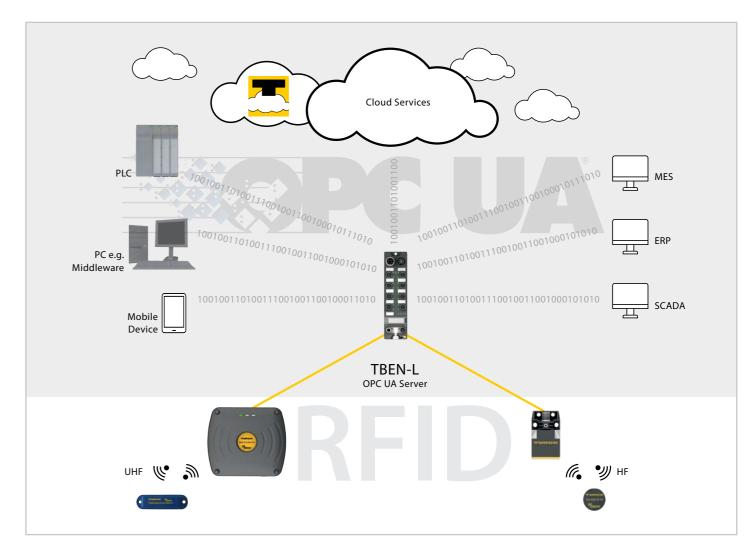
The TBEN-L5-4RFID-8DXP-OPC-UA with an integrated OPC UA server supports the connection of HF and UHF read/write heads as well as sensors and actuators. The
