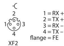
Fig. 7: Ethernet OUT pin assignment
