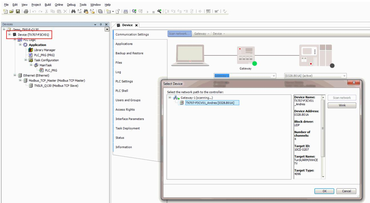
Fig. 19: Setting up a network interface to the Modbus master
