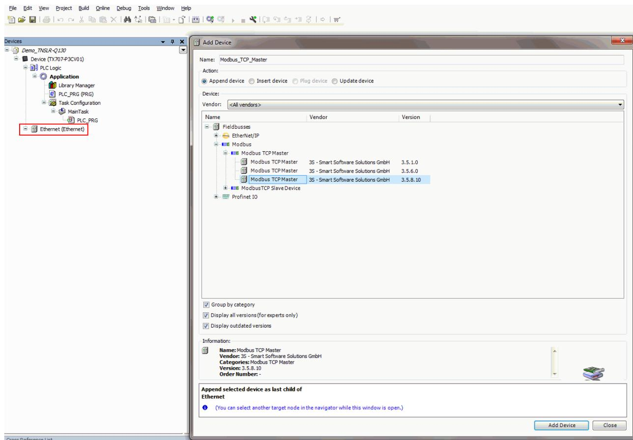
Fig. 16: Adding a Modbus master
