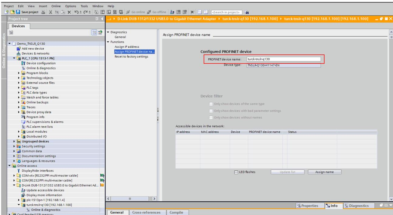
Fig. 36: Assigning the PROFINET device name
