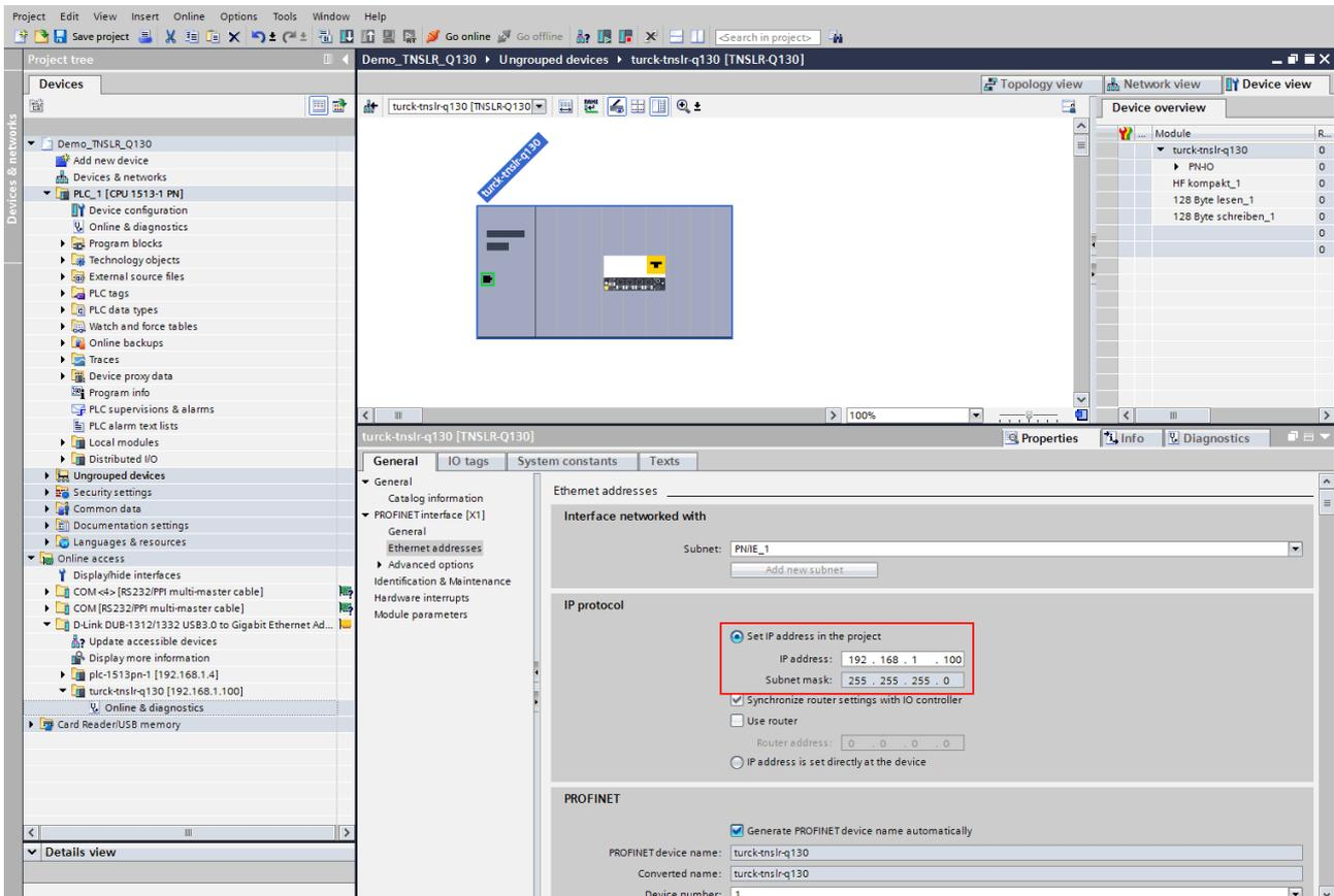
Fig. 37: Assigning the IP address
