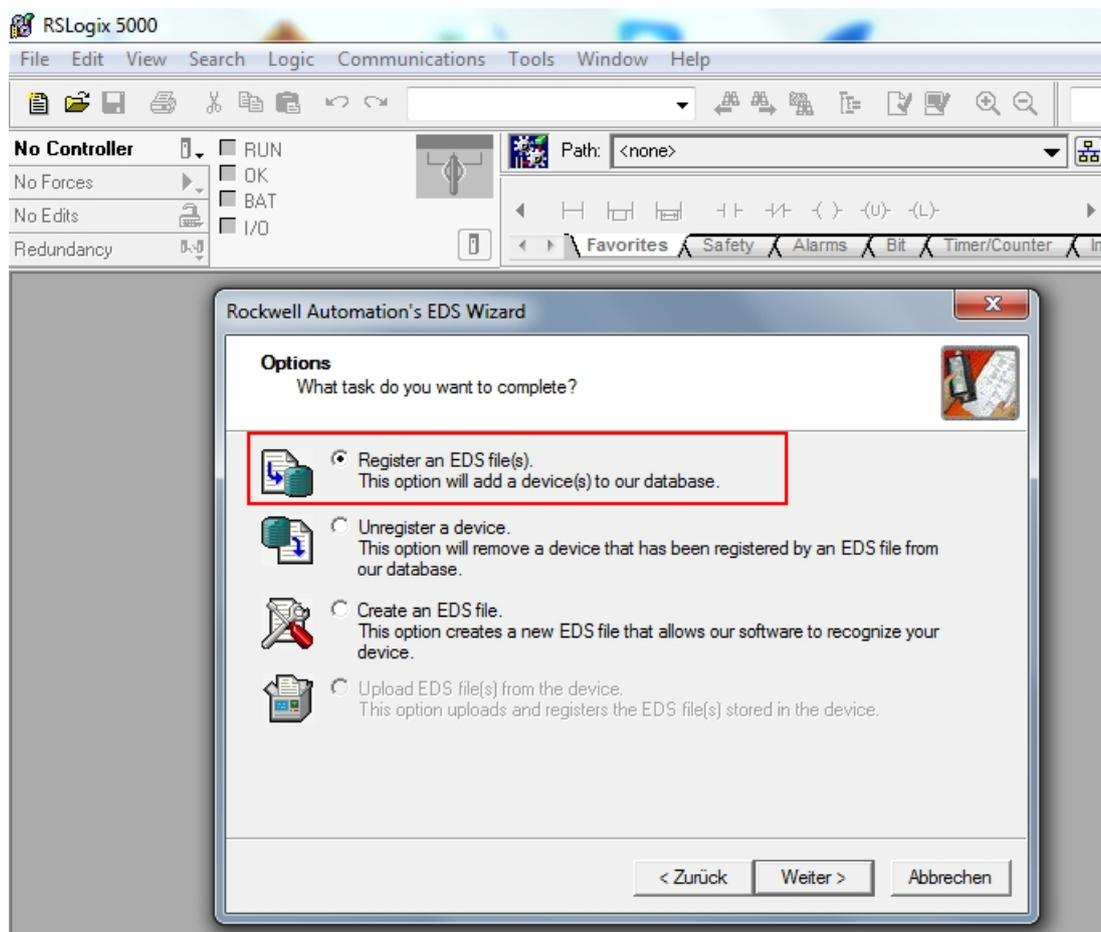
Fig. 28: Option selection — registering an EDS file(s)
