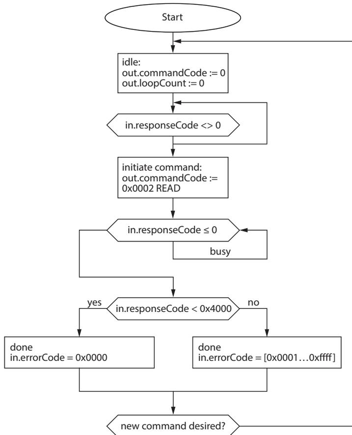
Fig. 55: Flow chart for command processing
