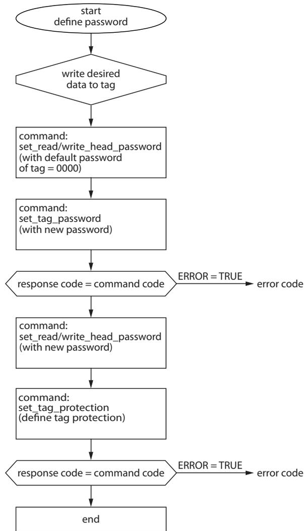
Fig. 60: programming tags with a password
