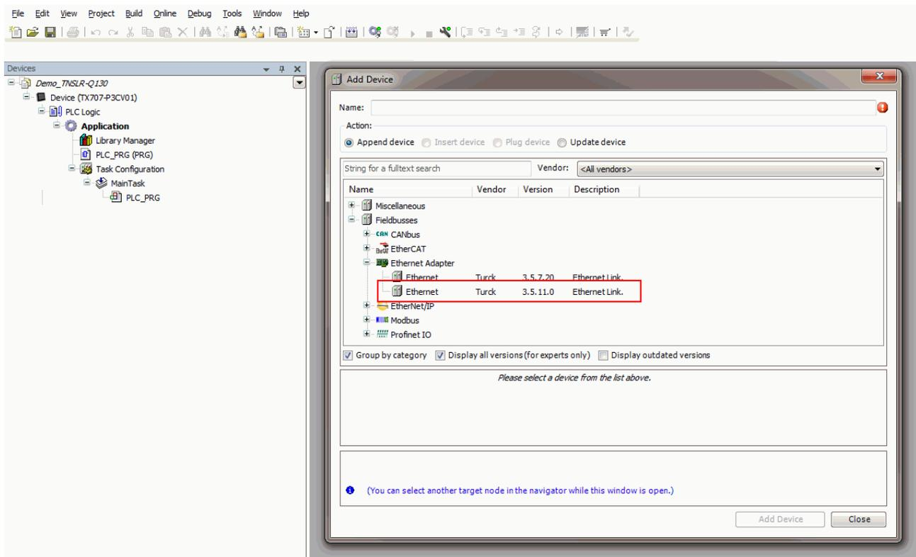
Fig. 15: Adding an Ethernet adapter
