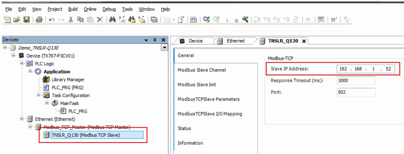
Fig. 21: Modbus slave – Entering the IP address (here: 192.268.1.52)
