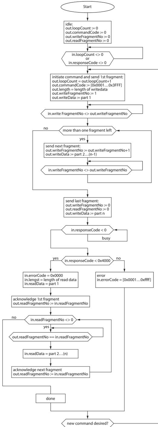
Fig. 57: Flow chart for command processing with fragmentation
