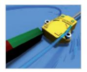
Robust housing – Made of high quality plastic. The IP67 rated sensor protects the sensor from most chemicals and oils. It is also shock and vibration resistant up to 30g's (11ms) and 55 Hz (1mm displacement).
