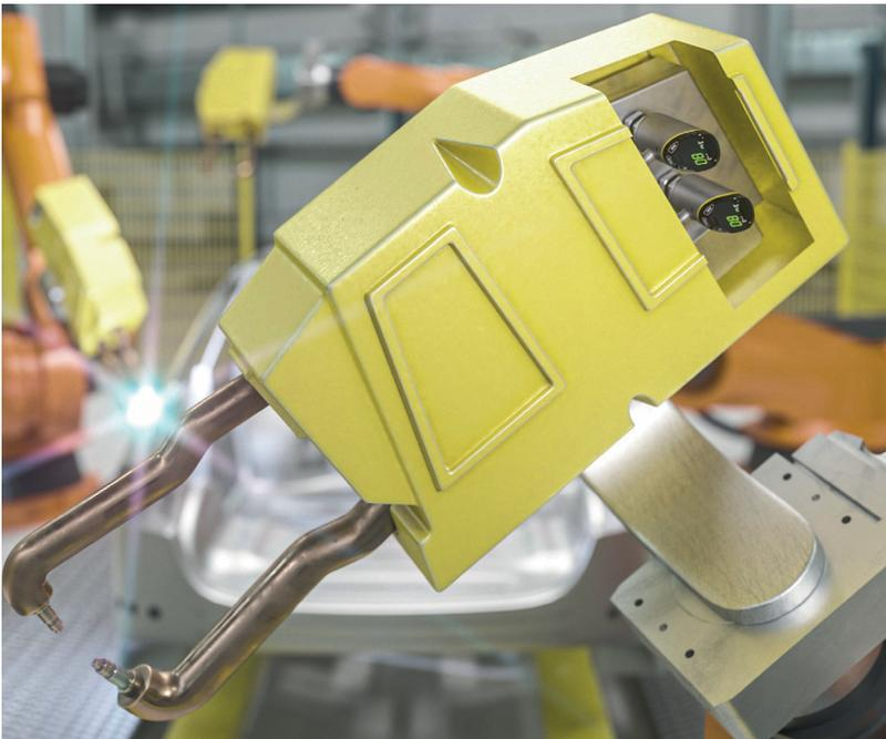
Monitoring the cooling circuit on welding clamps
