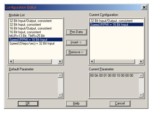
7 configurations are available for the regular operation of the encoder:
