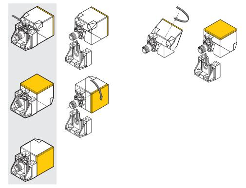
Fig. 10: Positioning the active face
