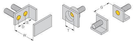
Fig. 8: Minimum mounting distances - Cylinder designs, flush mounting possible
