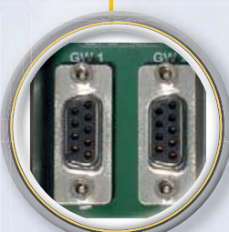
Connection of the higher-level PROFIBUS-DP fieldbus
