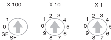
Figure 2: Setting the PROFIBUS-DP address
