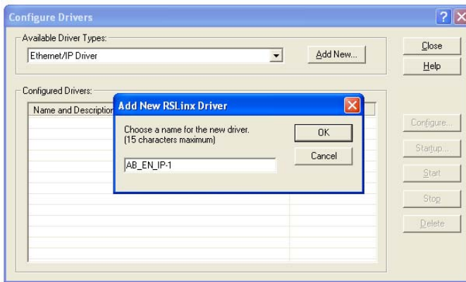
Figure 6-13: Selecting the EtherNet/IP Driver module
