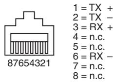
Fig. 5: RJ45 female connector
