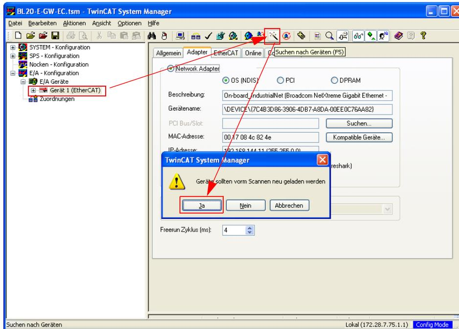
Fig. 10: Scanning the EtherCAT-network
