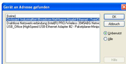
Fig. 9: Selecting the network interface card
