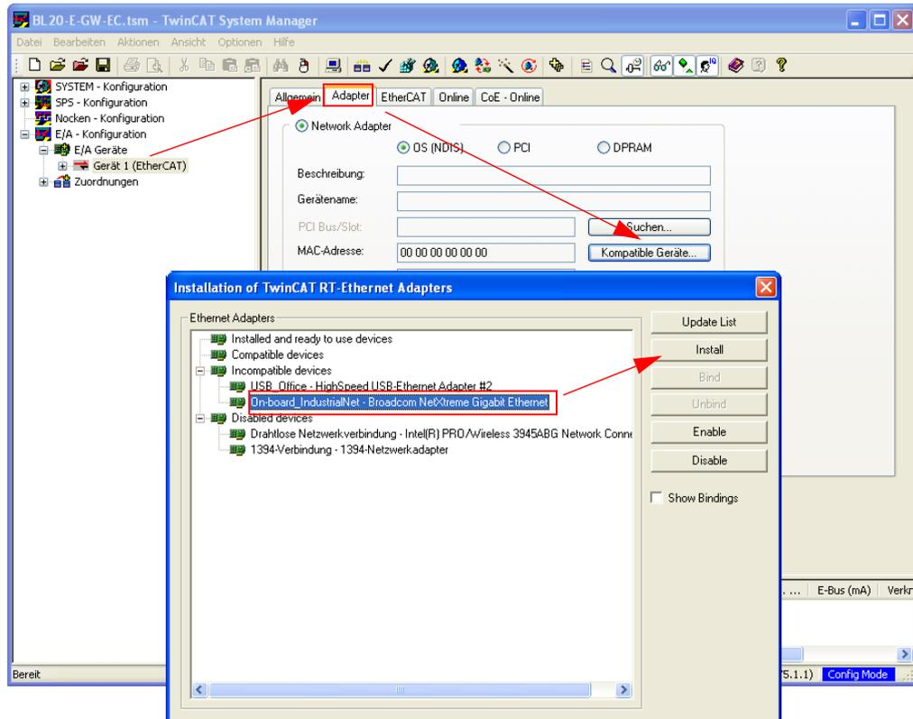
Fig. 28: Installation of the EtherCAT-driver
