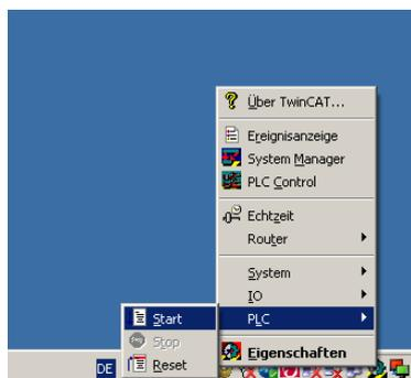
Fig. 17: Starting the PLC
