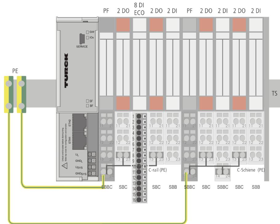
Fig. 38: Using the C-rail as a protective earth
