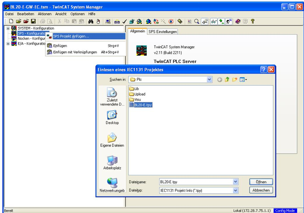
Fig. 19: Adding the PLC-program to the hardware-configuration.
