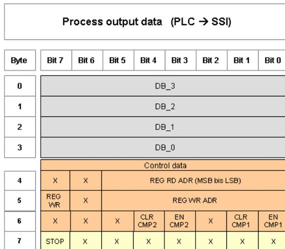
Fig. 34: Process output data
