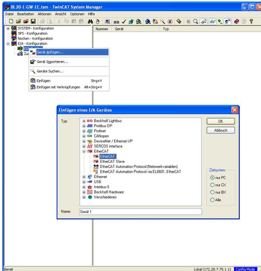
Fig. 8: Adding an EtherCAT-interface
