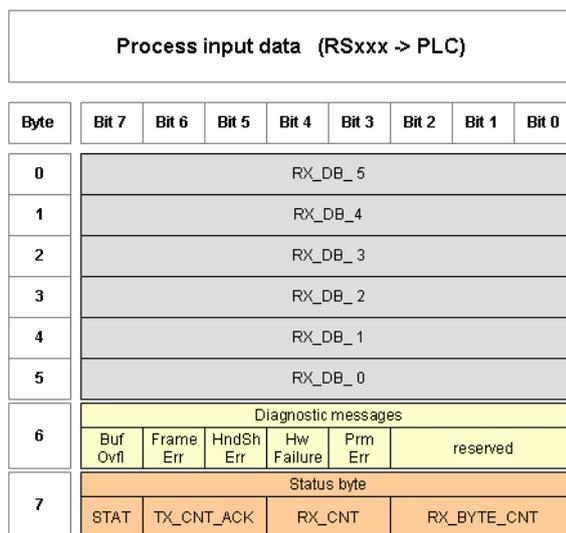
Fig. 29: Process input data SPS
