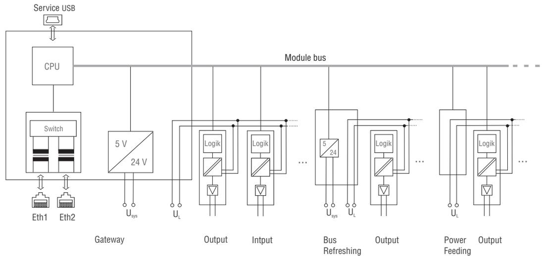
Fig. 40: Block diagram of a BL20 station with EtherCAT-gateway
