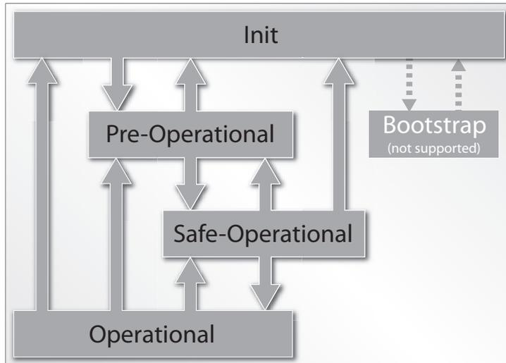
Fig. 1: EtherCAT-State Machine
