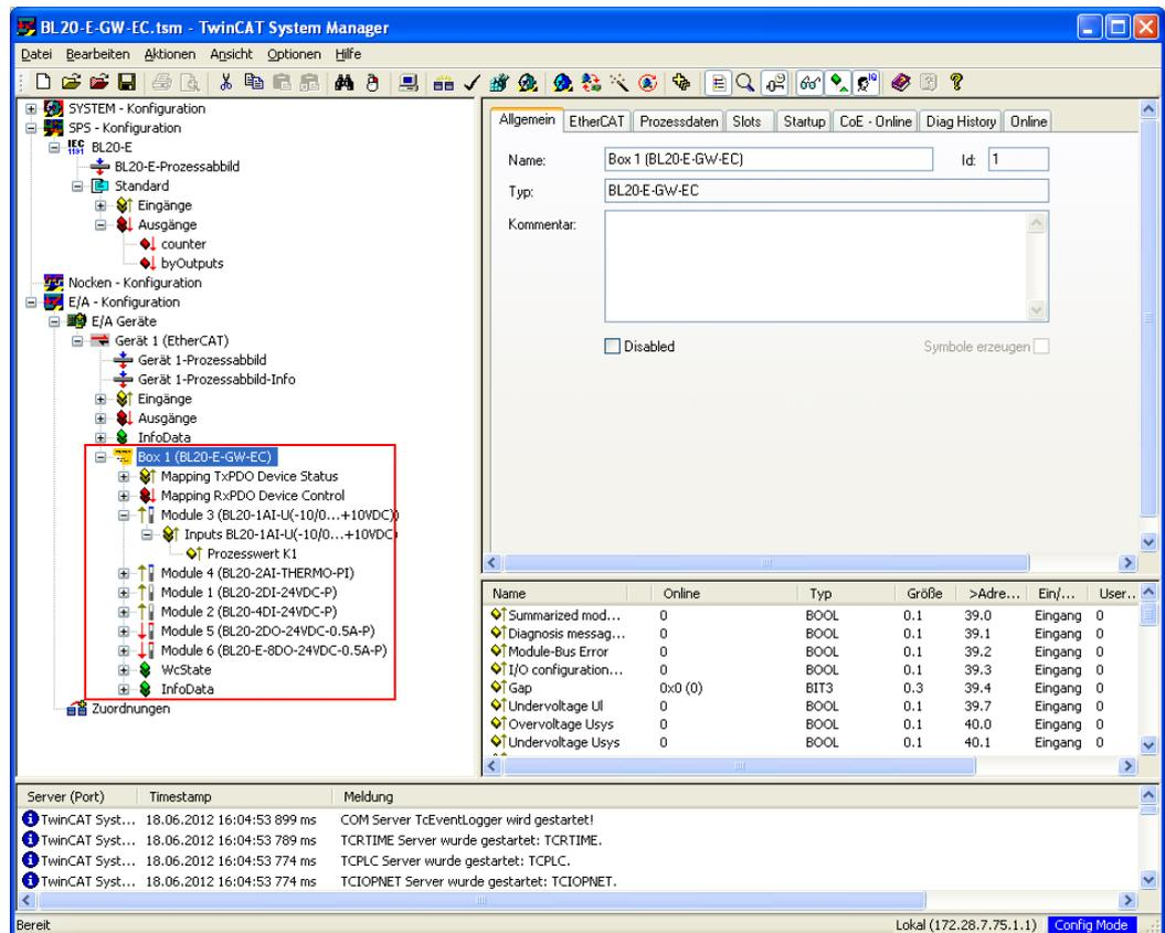
Fig. 11: BL20-station with \*.xml-file
