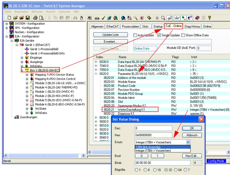
Fig. 13: Parameterization of a BL20-module
