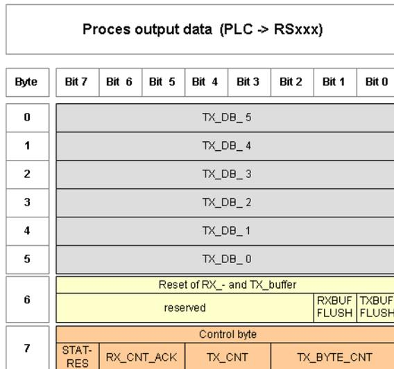
Fig. 32: Process output data SPS
