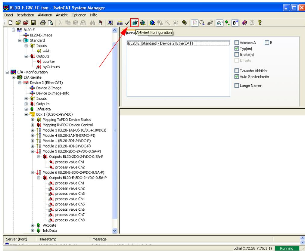
Fig. 23: Activate I/O-configuration
