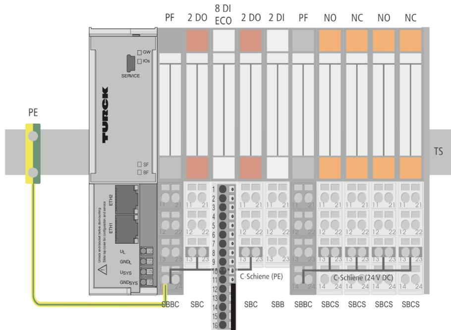
Fig. 39: Using the C-rail as protective earth and for the power supply with relay modules
