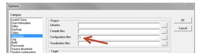
Add any .eds files to be used (in this case 'BLCCO-6M12L-4AI4AO-VI-2AO-I V1.22.eds') into the project folder. If any eds files are added in this manner, save & close then reopen the project.
