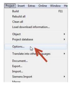
Select 'Directories' in the Category list. Be sure that in the configuration field '.\' is entered. Entering this causes CoDeSys to look in the local folder where the program is saved for any configuration files (.eds, .cfg, etc.), then load those files on program startup. This step would have likely been performed when setting up the CANopen Manager.
