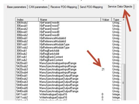
After all required values are entered, the PLC Configuration window can be closed. And the parameters will take effect next time the program is downloaded to the controller.
