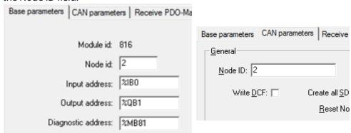
In this case, as we are configuring a node with analog inputs, it is important to configure the PDO communication parameters for Send PDOs that contain analog data (The default values CoDeSys uses would parameterize change-of-state transmission type. As this would overload the bus with analog data, the BLCCO would not transmit data on these PDOs.)
