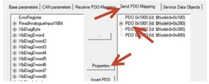
In the Properties window, in the 'Event time' field, enter a time value. This time value will be the delay between PDO transmissions for the particular Send-PDO chosen (therefore choose a logical value given data prioritization and bus characteristics). Then click 'OK' to close the window.
