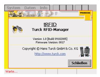
The splash screen includes important information on the software and hardware. The **Version** field shows the current version of tRFID together with the build code. The version and build code clearly identify a certain software development status. The **firmware version** indicates the version number of the loadable firmware in the RFID device.
