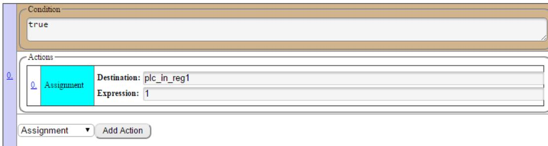
**Explaining the Code:** The user wrote the value “1” into plc\_in\_reg1.
