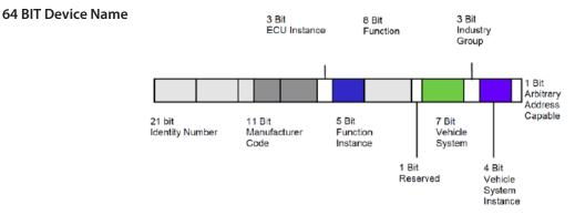
Since the function of a device is contained in the name, the address can be changed at will and the correct device is always addressed that provides the required functionality.
