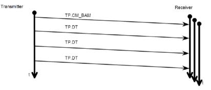
With the peer-to-peer transmission, the transmitter initiates the connection with a "request to send" message. The receiver then controls the transport protocol with "clear to send" and "end of message acknowledge."
