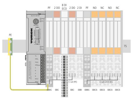
Fig. 27: Using the C-rail as protective earth and for the power supply with relay modules
