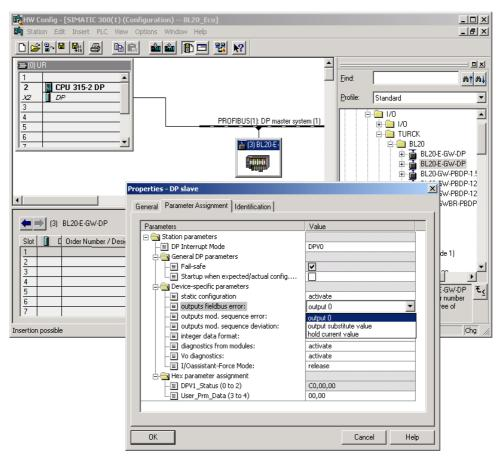
Fig. 13: Parameterization of the BL20-gateway
