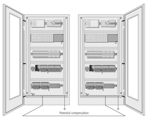
Fig. 32: Potential compensation between switchgear cabinets
