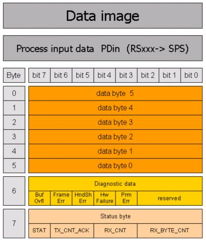
Fig. 39: Data image PLC input data
