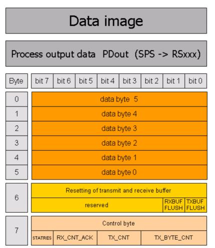
Fig. 40: Process output data
