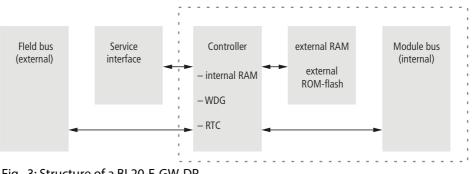
Fig.. 3: Structure of a BL20-E-GW-DP
