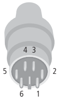
Figure 4-5: PS/2 male connector on the connection cable to the gateway (top view)
