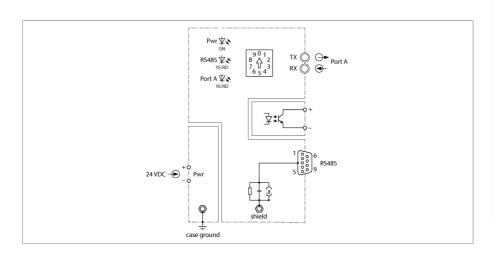
The FOC11... fiber optic media converter converts RS485 signals, e.g. from PROFIBUS-DP or Modbus RTU, on copper cables into optical signals and vice versa. Bus signals from the safe area up to zone 1 can thus be transmitted intrinsically safe, potential-free and interference-free over long distances.
