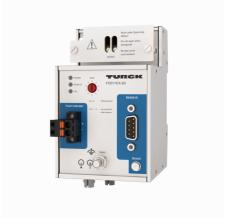
The FOC11... fiber optic media converter converts RS485-IS signals, e.g. from PROFIBUS-DP or Modbus RTU, on copper cables into optical signals and vice versa. Intrinsically safe bus signals from zone 1 can thus be transmitted intrinsically safe, potential-free and interference-free over long distances.
