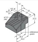
Floating positioning element for linear position sensors LI-Q25L; the nominal distance to the sensor is 1.5 mm; pairing with the linear position sensor at a distance of up to 5 mm or misalignment tolerance of up to 4 mm.
