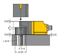
Ri-DSU35 for mounting on rotary actuators The Ri-DSU35 angle sensor and the well-established Ni4-DSU35 inductive dual sensor are identical in construction. The user also profits from the enormous mounting flexibility of the device. The sensor can be mounted on all standard rotary actuators with a shaft diameter of max.14 mm thanks to an extensive range of available accessories. For larger shaft diameters use the BTS-DSU35-Z02 accessories.
