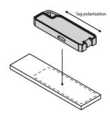
The tag is delivered with an adhesive strip on the underside and can be applied at an ambient temperature of 21 °C to 38 °C.
