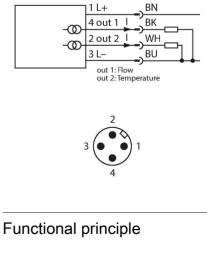
The flow sensor functions according to the calorimetric principle. The distinctive feature of this principle is that the flow rate correlates directly to the thermal loss of energy in
