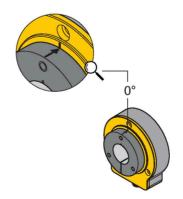
The extensive range of mounting accessories enables easy adaptation to many different shaft diameters. Due to the measuring principle, which is based on the functional principle of an RLC coupling, the encoder is immune to magnetized ferrous chips and other interferences. As a result, there are few possible causes of error during mounting. The adjacent figures show the simple installation of the two separate units: the sensor element and the positioning element: Mounting option A:
