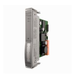
The PSM24... power supply module supplies the excom system with power to the full extension. The power supply module can be used in Zone 2.
