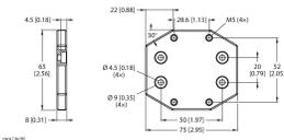
Adapter plate for mounting the QR20 housing with mounting holes for the Q20L60 housing
