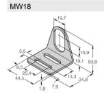
Mounting bracket for threaded barrel sensors; material: Stainless steel A2 1.4301 (AISI 304) BSS-18
