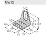
6945003 Mounting bracket for threaded barrel sensors; material: Stainless steel A2 1.4301 (AISI 304)
