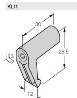
Mounting bracket for mounting magnetic field sensors on tie-rod cylinders; cylinder diameter: 32...100 mm; material: Die-cast Zinc
