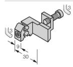
Mounting bracket for mounting magnetic field sensors on profile cylinders with external dovetail guide; cylinder diameter: 32...200 mm; material: Aluminum
