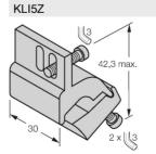
6971803 Mounting bracket for mounting magnetic field sensors on tie-rod cylinders; cylinder diameter: 32...63 mm; material: Aluminum
