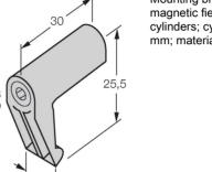
Mounting bracket for mounting magnetic field sensors on tie-rod cylinders; cylinder diameter: 32...100 mm; material: Die-cast Zinc
