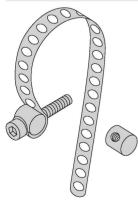
Mounting on round cylinders; cylinder diameter 80...200 mm material: Metal A2 1.4301 (AISI 304); two tie bolts (material: Metal CuZn, alternatively metal A2 1.4301 / AISI 304) cylinder screw M3 x 20; (DIN 912-A20)
