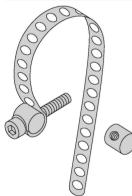
69653 Mounting on round cylinders; cylinder diameter 8...25 mm; material: Metal CuZn; two tie bolts (material: Metal CuZn), cylinder screw M3 x 20
