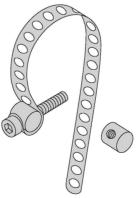
Mounting on round cylinders; cylinder diameter 80...200 mm material: Metal A2 1.4301 (AISI 304); two tie bolts (material: Metal CuZn, alternatively metal A2 1.4301 / AISI 304) cylinder screw M3 x 20; (DIN 912-A20)
