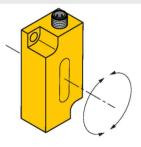
Adjusting the measuring range via TX1-Q20L60 teach adaptor
