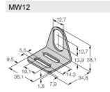
6945003 Mounting bracket for threaded barrel sensors; material: Stainless steel A2
