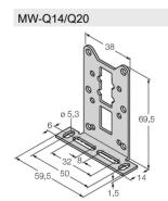
6945006 Mounting bracket for rectangular Q14 or Q20; material VA 1.4301
