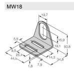
6945004 Mounting bracket for threaded barrel sensors; material: Stainless steel A2 1.4301 (AISI 304)
