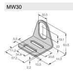
6945005 Mounting bracket for threaded barrel sensors; material: Stainless steel A2 1.4301 (AISI 304)
