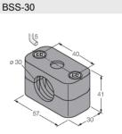
Mounting clamp for smooth and threaded barrel sensors; material: Polypropylene
